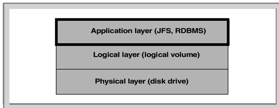
Figure 102. LVM components, the application layer
