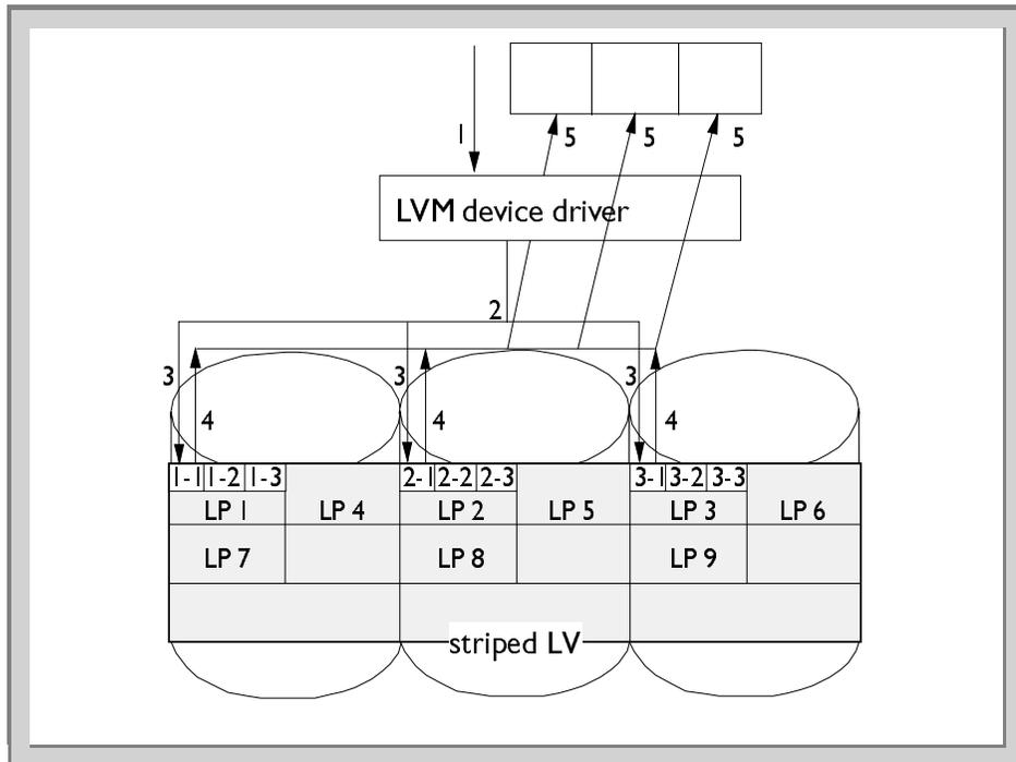
Figure 49. The striped logical volume: The read phase
