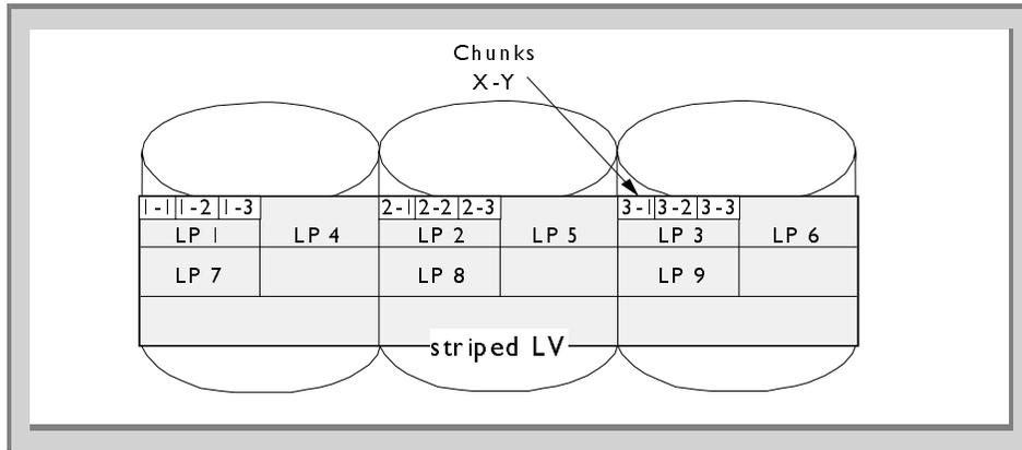
Figure 47. Physical partitions are divided into many chunks
