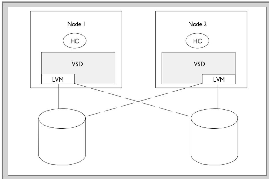
Figure 73. Concept of the Recoverable Virtual Shared Disk
