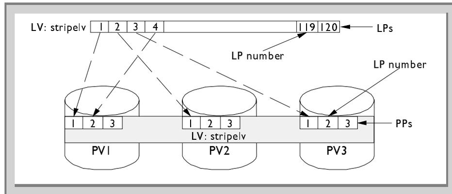
Figure 46. The striped logical volume - Physical partition mapping
