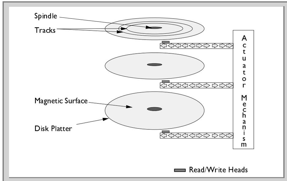
Figure 4. The structure of a disk drive
