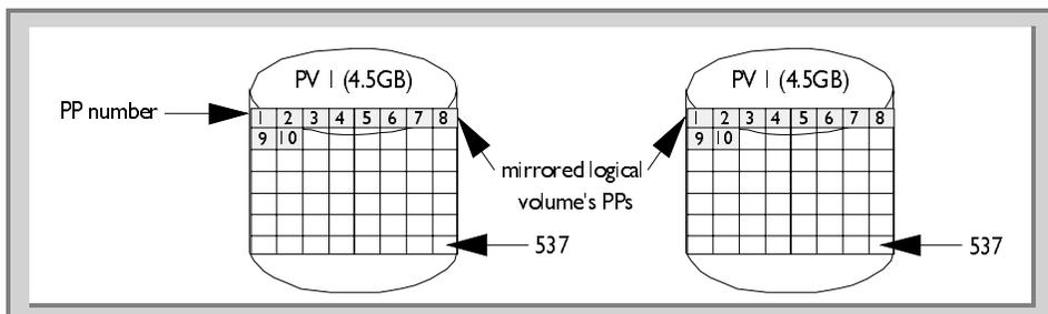
Figure 32. Exact mapping - Physically identical allocation
