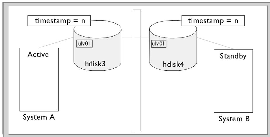
Figure 12. Two systems sharing two disks; system A is active.
