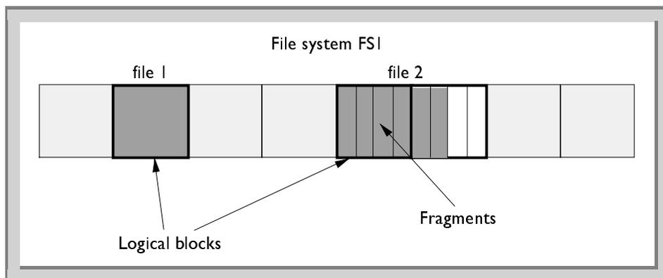
Figure 79. Logical blocks and fragments partially filled
