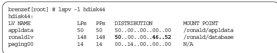
Looking at the logical volume name `ronaldlv`, you see that 50 physical partitions are located on the outer edge and 46 and 52 on the inner-middle and the inner edge.
