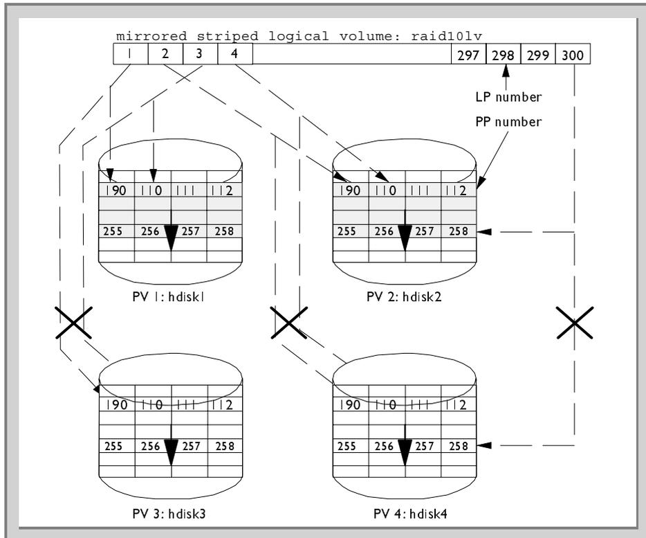
Figure 64. Removal of one mirror from the mirrored and striped logical volume
