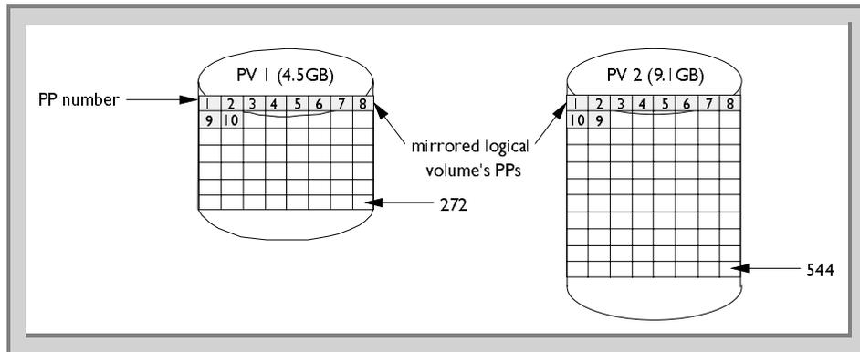
Figure 31. Exact mapping - Logically identical allocation
