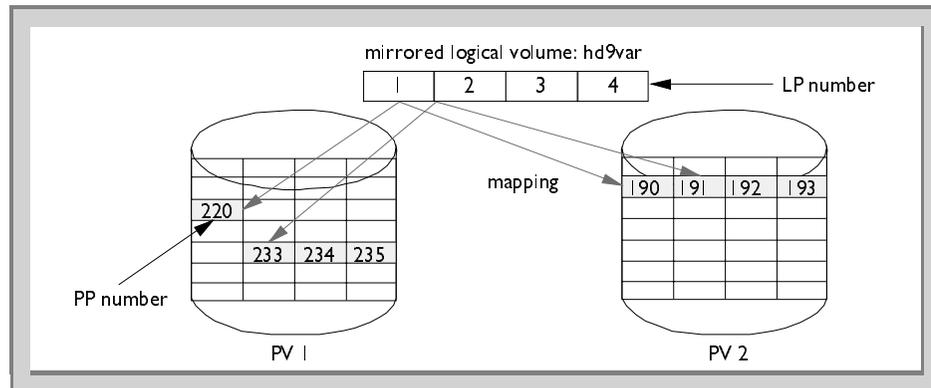
Figure 25. Mapping - Relationship between logical partition and physical partitions
