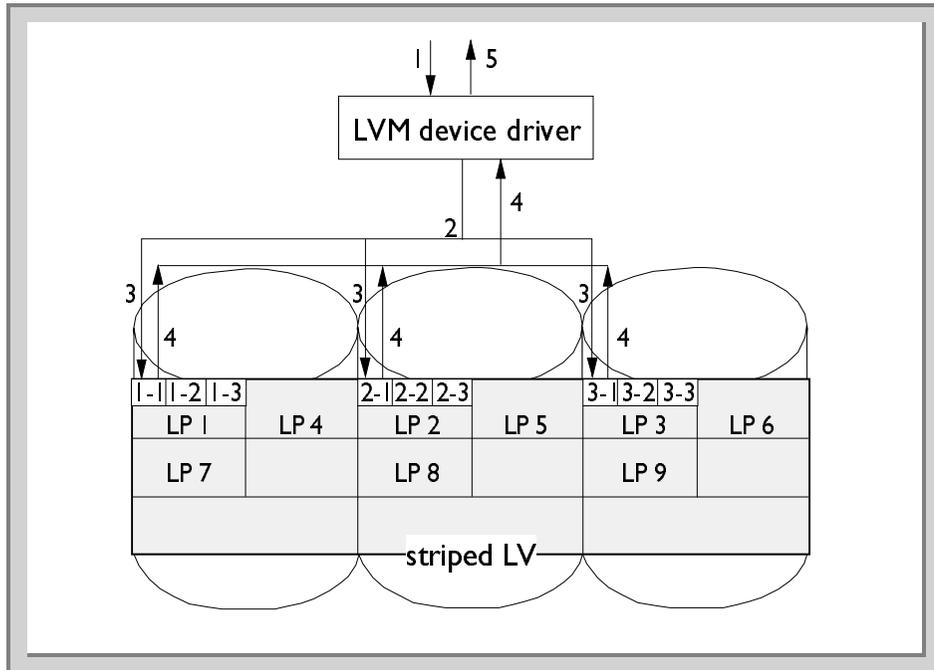
Figure 48. The striped logical volume - Write phase behavior
