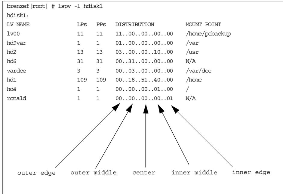
Figure 101. Example of a disk distribution
