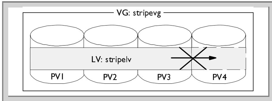
Figure 53. Impossible extension of the striped logical volume
