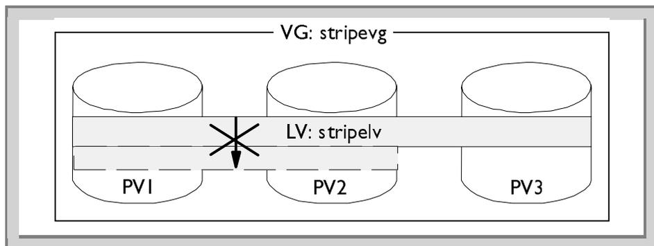
Figure 54. Impossible extension of the striped logical volume with wrong width
