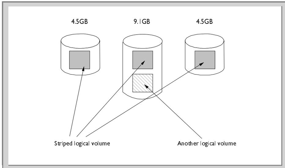
Figure 100. Striping on different size disks with extra logical volume
